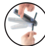
Speed and ease of use: position the sheath-stripper. Turn around the cable. Pull outwards.
