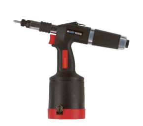
Hydraulic/pneumatic blind rivet nut tool with automatic right and left hand running. Including quick interchange system. For correct deformation of the blind rivet nut/-bolt, an air pressure regulator is build in.
